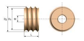
Thread fitting for assembly in tension spring coils, see previous pages. This fitting is safer than conventional loops, which is why higher loads are permitted on the spring. The coil can be cut into the required length, and the fitting can be mounted without any special tools.
